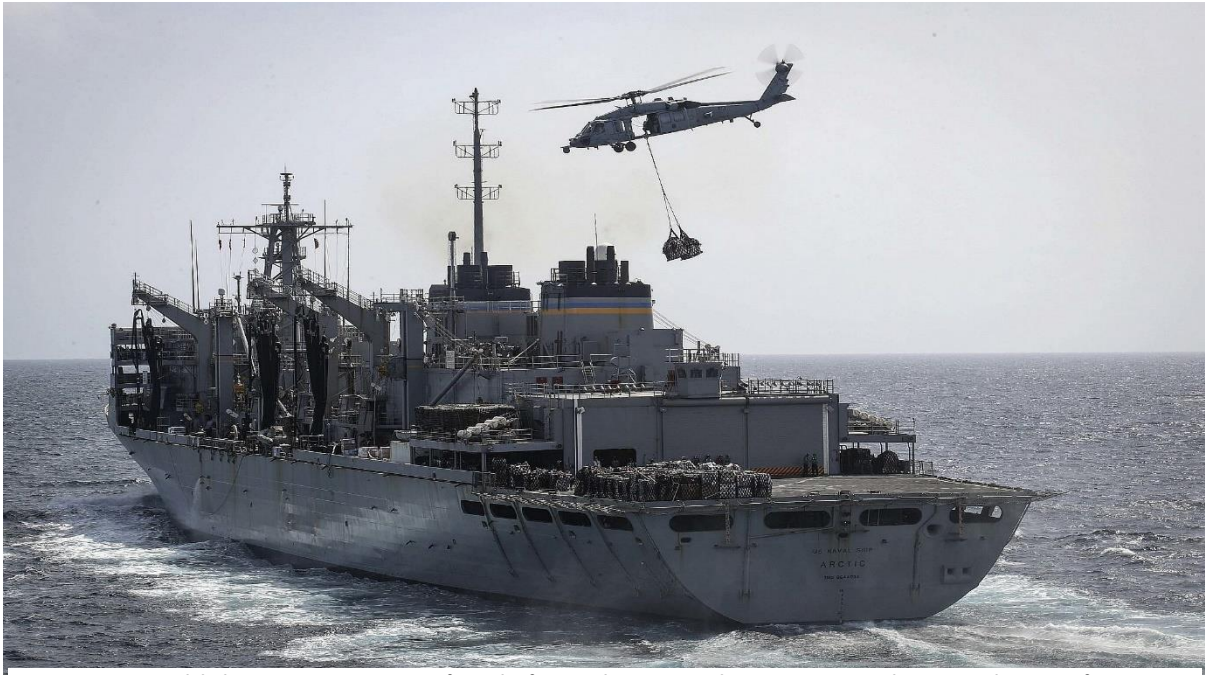
an MH-60S Sea Hawk helicopter transports cargo from the fast combat support ship USNS Arctic to the Nimitz-class aircraft carrier USS Abraham Lincoln during a replenishment-at-sea in the Arabian Sea [AP]
